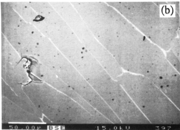
Figure 3. Electron microprobe micrographs of (a) La_{0.8}Ba_{0.2}TiO_3 (interior of melt) and (b) La_{0.8}Ba_{0.2}TiO_3 (exterior of melt). The scale given in the lower left corner of each micrograph is 50 \mu m .
